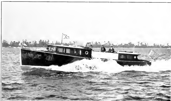
Cora S. III of West Palm Beach, designed by Henry C. Grebe & Co., and built by Great Lakes Boat Building Corp.; 46 feet long and powered with twin Sterling Petrel 6-cylinder engines rated 200 horsepower. At 2000 revolutions per minute she makes a maximum speed of 28 miles and a cruising speed of 25 miles per hour. At the right is shown the very neat engine installation and the throttle control from the navigating bridge.
